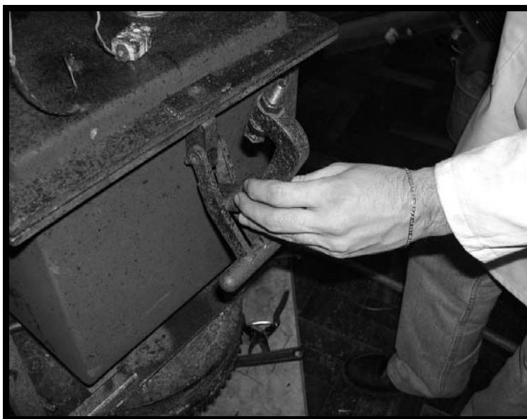
Figure 1.17c Clamping of mould
