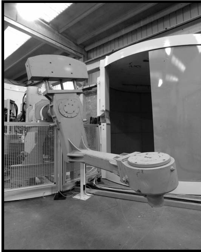
Figure 3.14 A typical drop arm Courtesy of Polivinil Rotomachinery SpA
