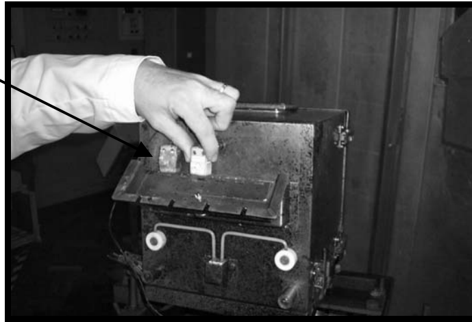
Figure 3.28 Thermocouples being attached to Rotolog
