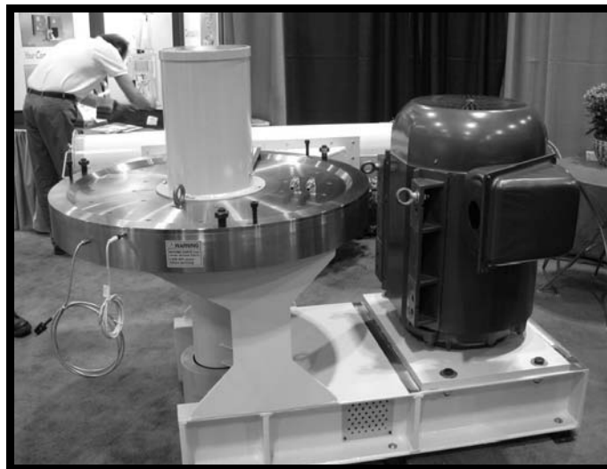
Figure 4.21 Horizontal grinding head
