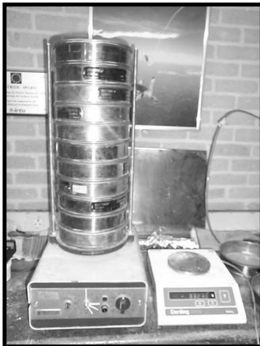
Figure 4.24 Typical sieve shaker used for rotational moulding powders
