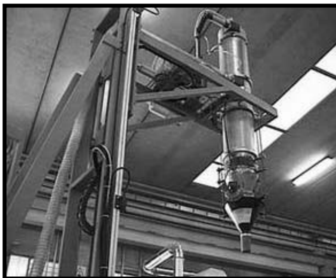
Figure 2.22 Automatic material dispenser Courtesy of Persico SpA
