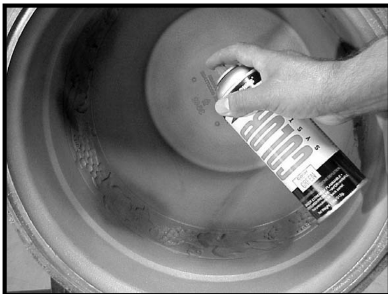
Figure 5.16 In mould colour spray Courtesy of Mold In Graphic Systems®
