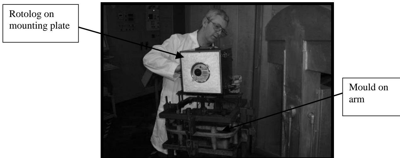
Figure 3.26 Rotolog being attached to mounting bracket
