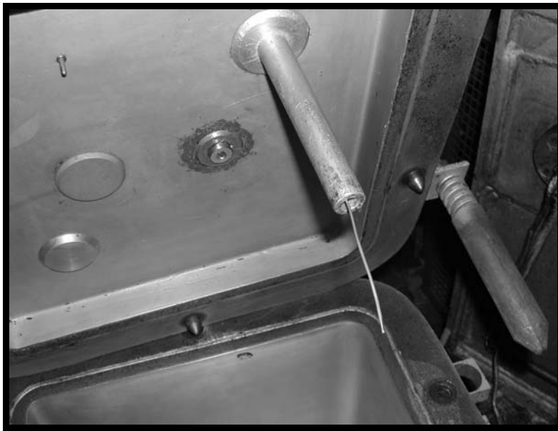
Figure 3.40 Thermocouple extending through vent tube
