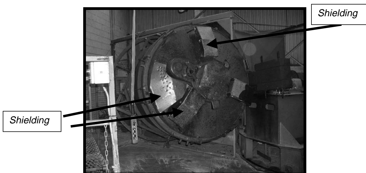
Figure 5.2 Tank with shielding on lid Courtesy of Clarehill Plastics Limited
