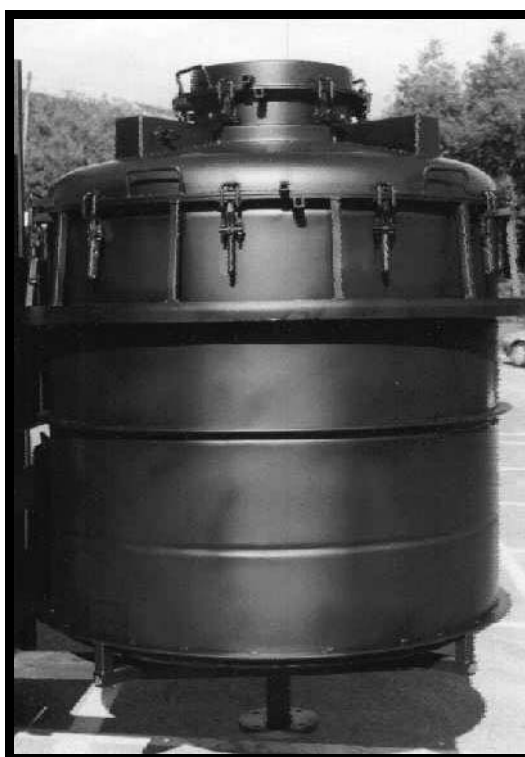
Figure 2.1 Sheet metal mould for a vertical tank
