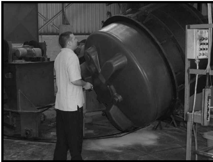
Figure 1.17l Final part removal from mould Courtesy of Clarehill Plastics Limited
