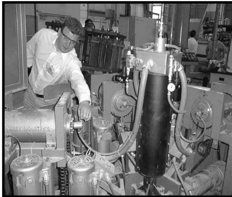
Figure 3.35 Air passed to rotary couplings
