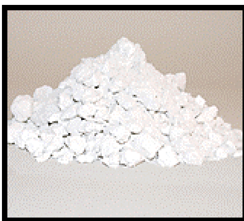
Figure 4.9 Calcium carbonate filler
