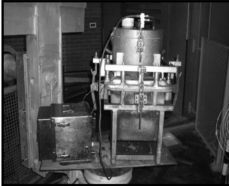
Figure 4.11a Drop box on mould
