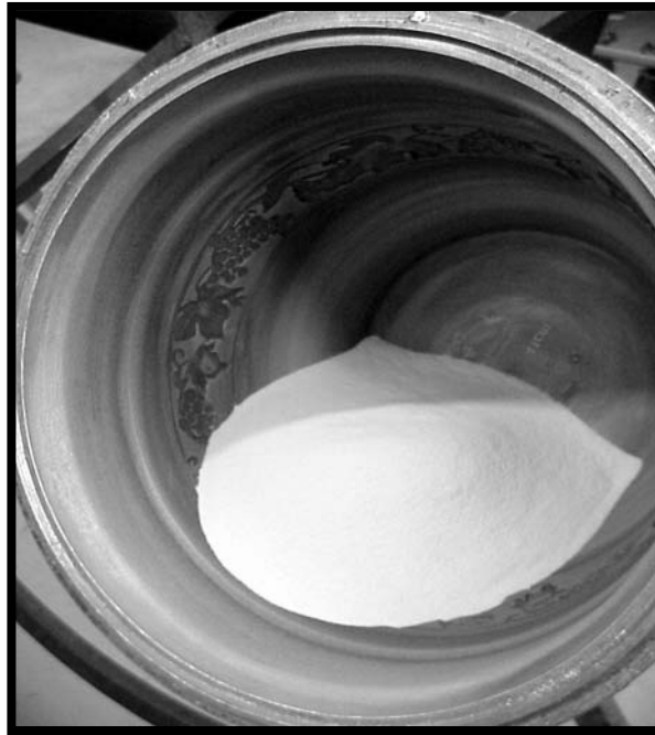
Figure 5.17 PE powder placed in mould Courtesy of Mold In Graphic Systems®
