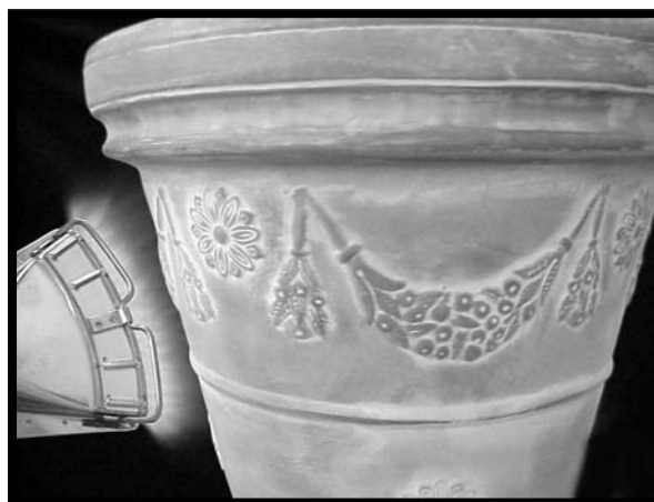
Figure 5.12 Final flame treatment Courtesy of Mold In Graphic Systems®
