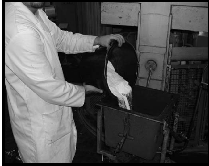
Figure 1.17a Operator begins charging mould
