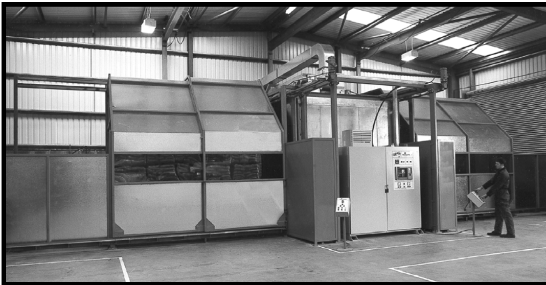
Figure 3.4 Two station shuttle machine with cooler bay doors Courtesy of Ferry Industries Inc.
