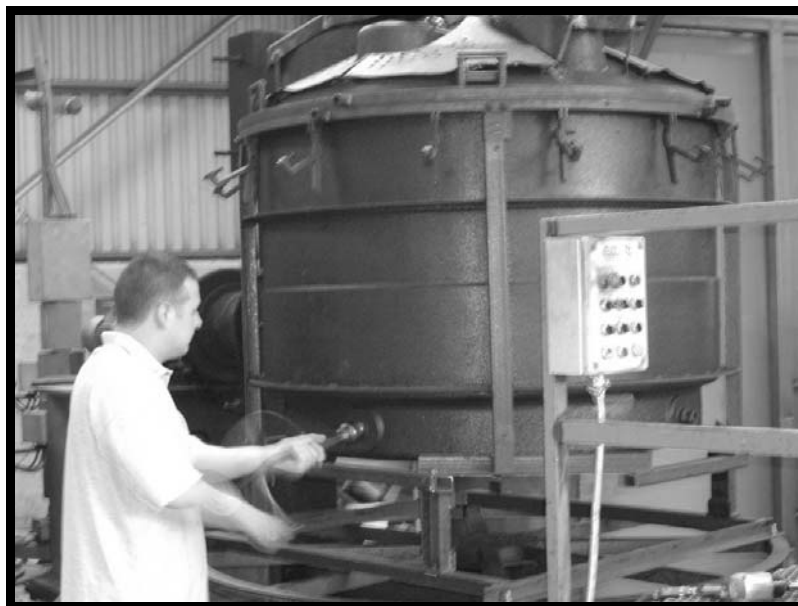
Figure 1.17j Removal of mould-in insert holder Courtesy of Clarehill Plastics Limited
