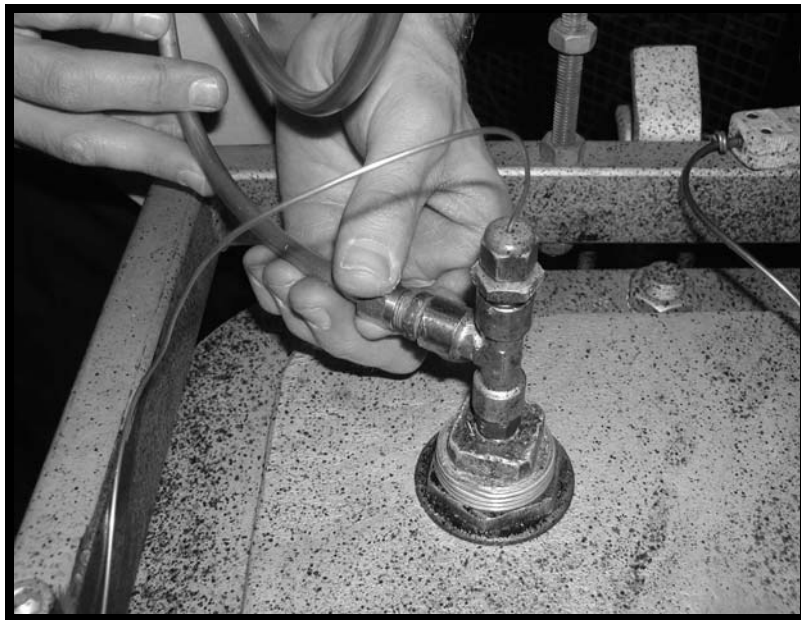
Figure 3.39 Mould attachment for air line and thermocouple
