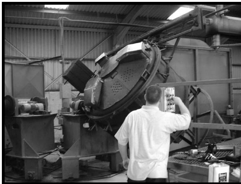
Figure 1.17i Mould in demoulding bay being rotated into a convenient orientation to assist demoulding Courtesy of Clarehill Plastics Limited
