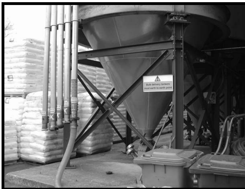
Figure 4.15 Granule feed system
