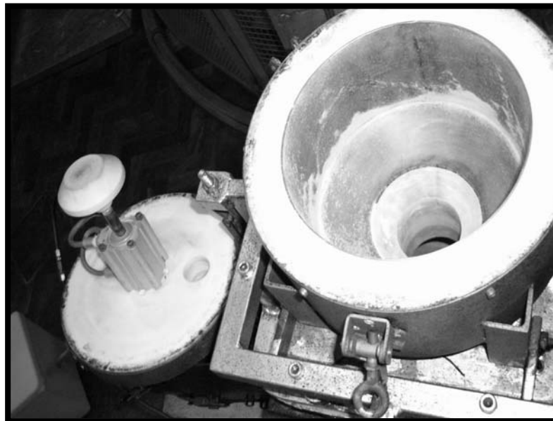
Figure 4.11b Drop box on mould, open showing valve position
