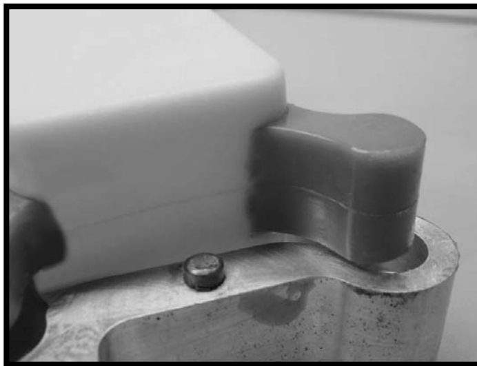
Figure 2.24d Final moulding contains solid protrusion Courtesy of Mold In Graphic Systems®
