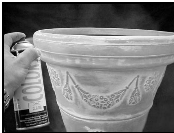
Figure 5.11 Paint sprayed onto moulded part Courtesy of Mold In Graphic Systems®
