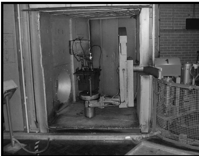
Figure 1.17f Arm with mould & Rotolog™ moving into oven
