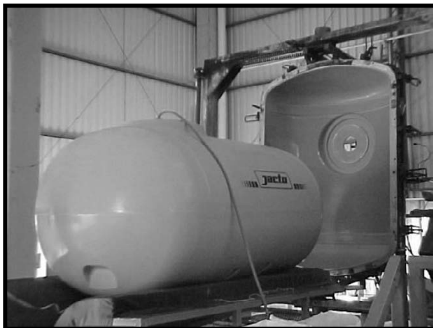
Figure 5.14 Graphic in place following demoulding Courtesy of Mold In Graphic Systems®
