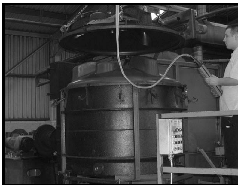
Figure 1.17k Lid removal using a crane Courtesy of Clarehill Plastics Limited
